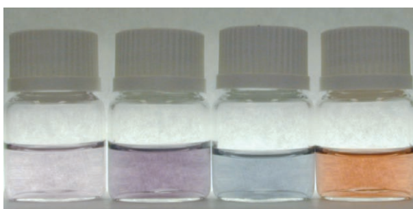
Figure 1. Photograph of suspensions of colloidal gold particles in H 2 O/EtOH 1:1, which were formed in the presence of (from left to right) no CB, CB[5], CB[6], and CB[7].
